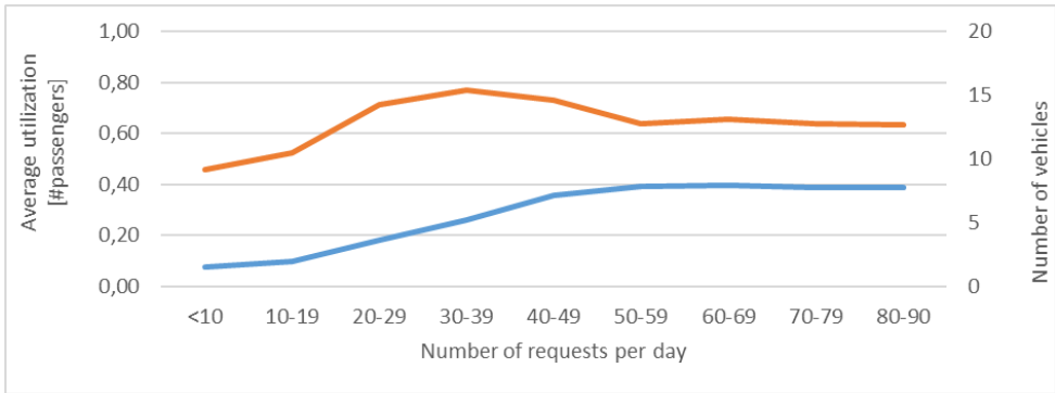
Figure 22. Average utilisation (orange line) and number of vehicles (blue line) depending on the number of requests.
