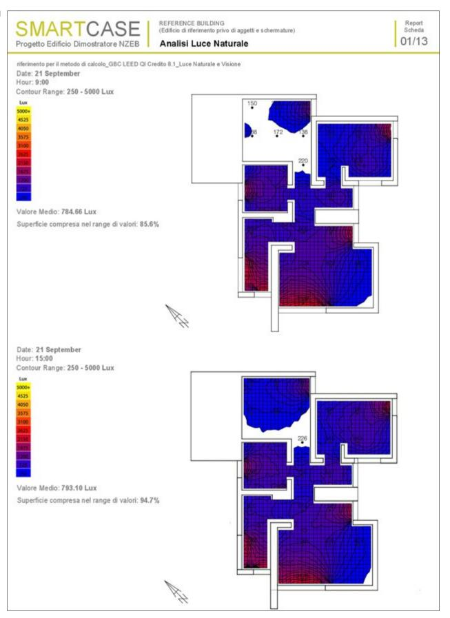
02 | Simulations for the optimization of the relationship between the shape of the building and the levels of natural lighting and reduction of the thermal load on the transparent envelope
