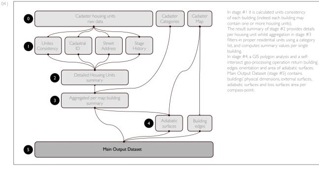
04 | Geo-DBMS multi-stage processing procedure
