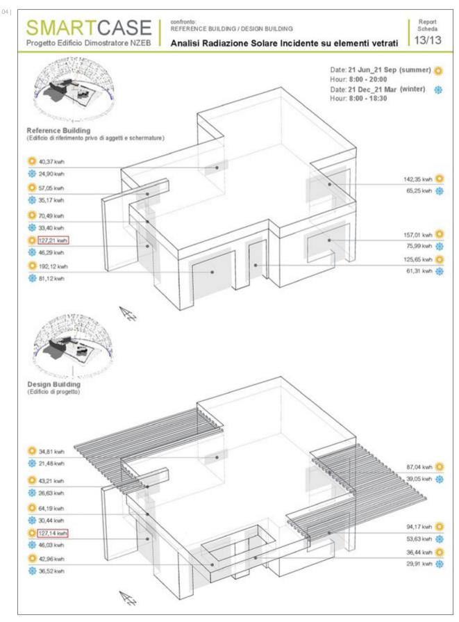
04 | Simulations for the optimization of the relationship between the shape of the building and the levels of natural lighting and reduction of the thermal load on the transparent envelope
