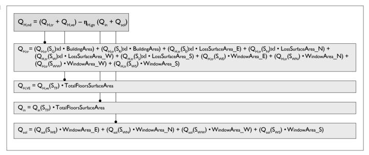
07 | Formula utilized in the GIS environment to calculate the annual heating energy demand for each building; the formula merges energetic data of the Dynamic Energy Simulations (Figure 6) with geometric data of buildings (Figure 5)
