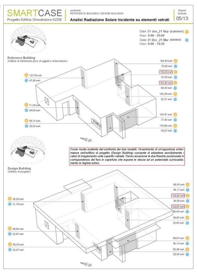
03 | Simulations for the optimization of the relationship between the shape of the building and the levels of natural lighting and reduction of the thermal load on the transparent envelope
