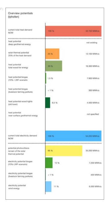
07 | Overview of the energy potentials (lphofen) which cover the electricity requirement, assisted by cogeneration plants dedicated to producing thermal energy for heat and sanitary hot water, as well as to covering any peaks in electricity demand. The thermal energy requirement for cooling, on the other hand, is guaranteed by heat exchangers deployed in specific, known points for extremely low temperatures, even in the summer period (BSUG, 2011).
